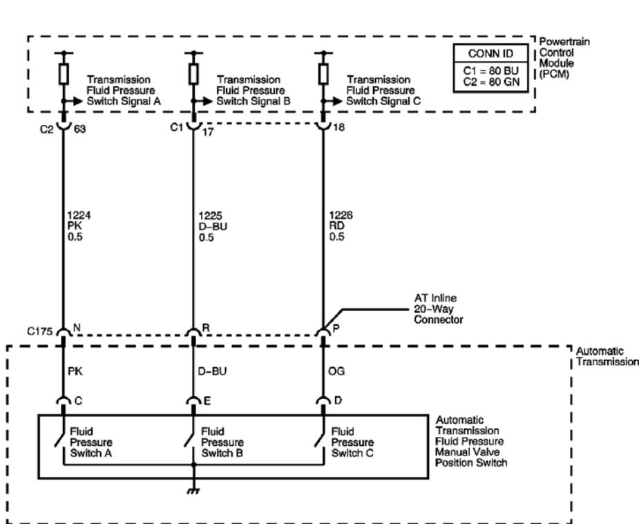
**Fig. 22: Automatic Transmission Fluid Pressure (TFP) Manual Valve Position Switch Diagram**
