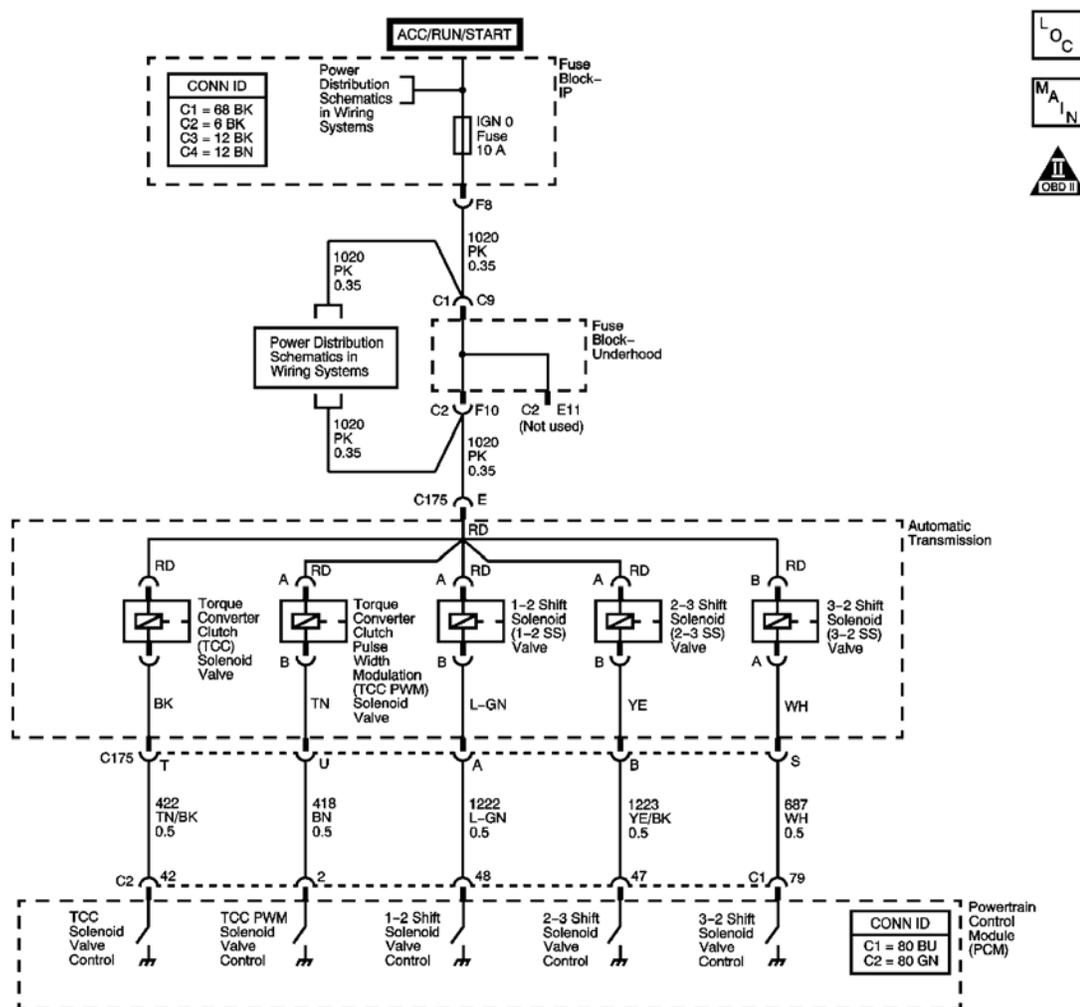
**Fig. 23: Torque Converter Clutch Pulse Width Modulation (TCC PWM) Solenoid Valve Diagram**
