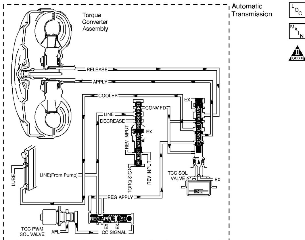
**Fig. 12: Torque Converter Clutch (TCC) Fluid Diagram**
