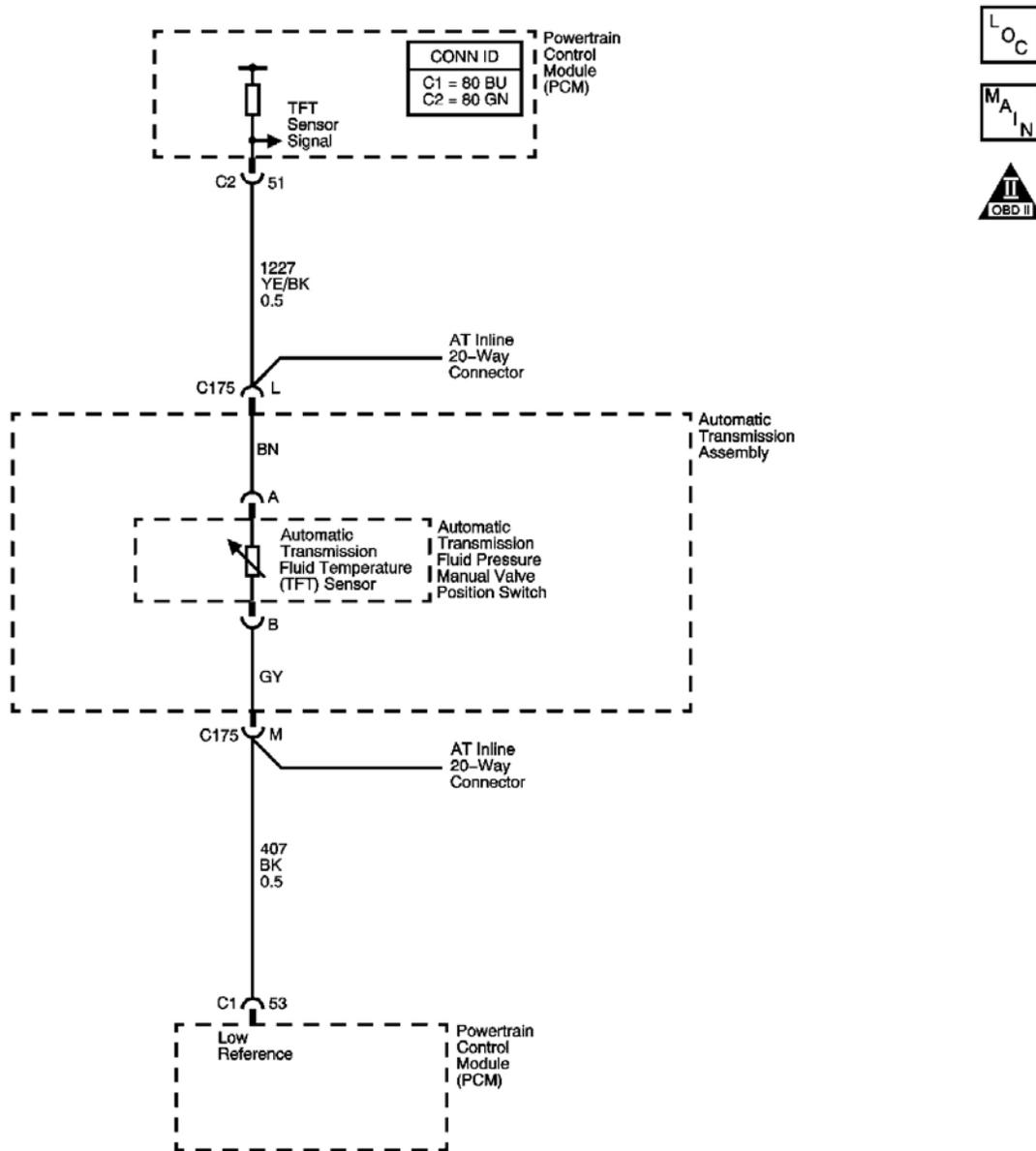
**Fig. 6: Automatic Transmission Fluid Temperature (TFT) Sensor**
