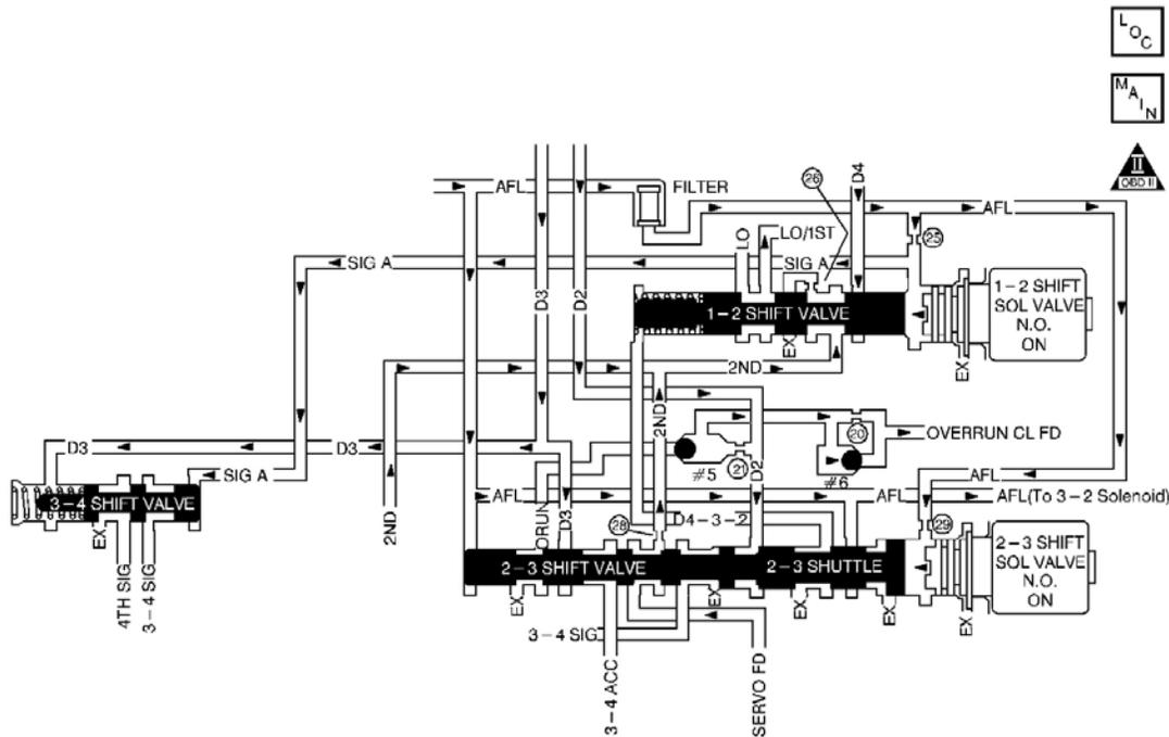
**Fig. 17: 1-2 Shift Solenoid (SS) & 2-3 Shift Solenoid (SS) Valve Fluid Diagram**
