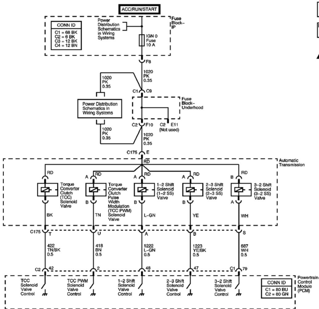
**Fig. 16: 1-2 Shift Solenoid (SS) Valve Diagram**
