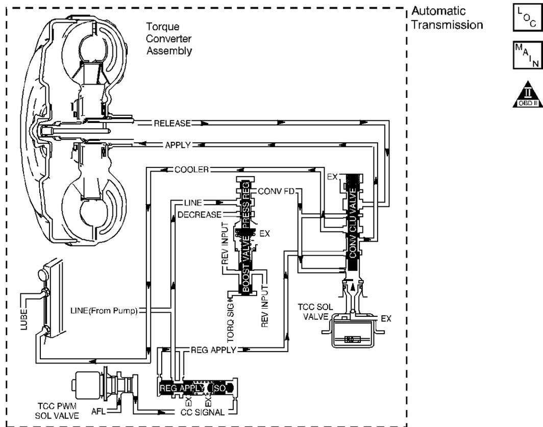
**Fig. 11: Torque Converter Clutch (TCC) Fluid Diagram**
