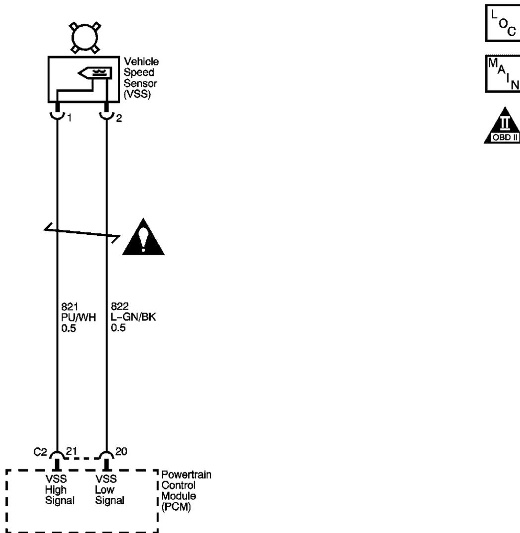
**Fig. 3: Vehicle Speed Sensor (VSS) Assembly Diagram**
