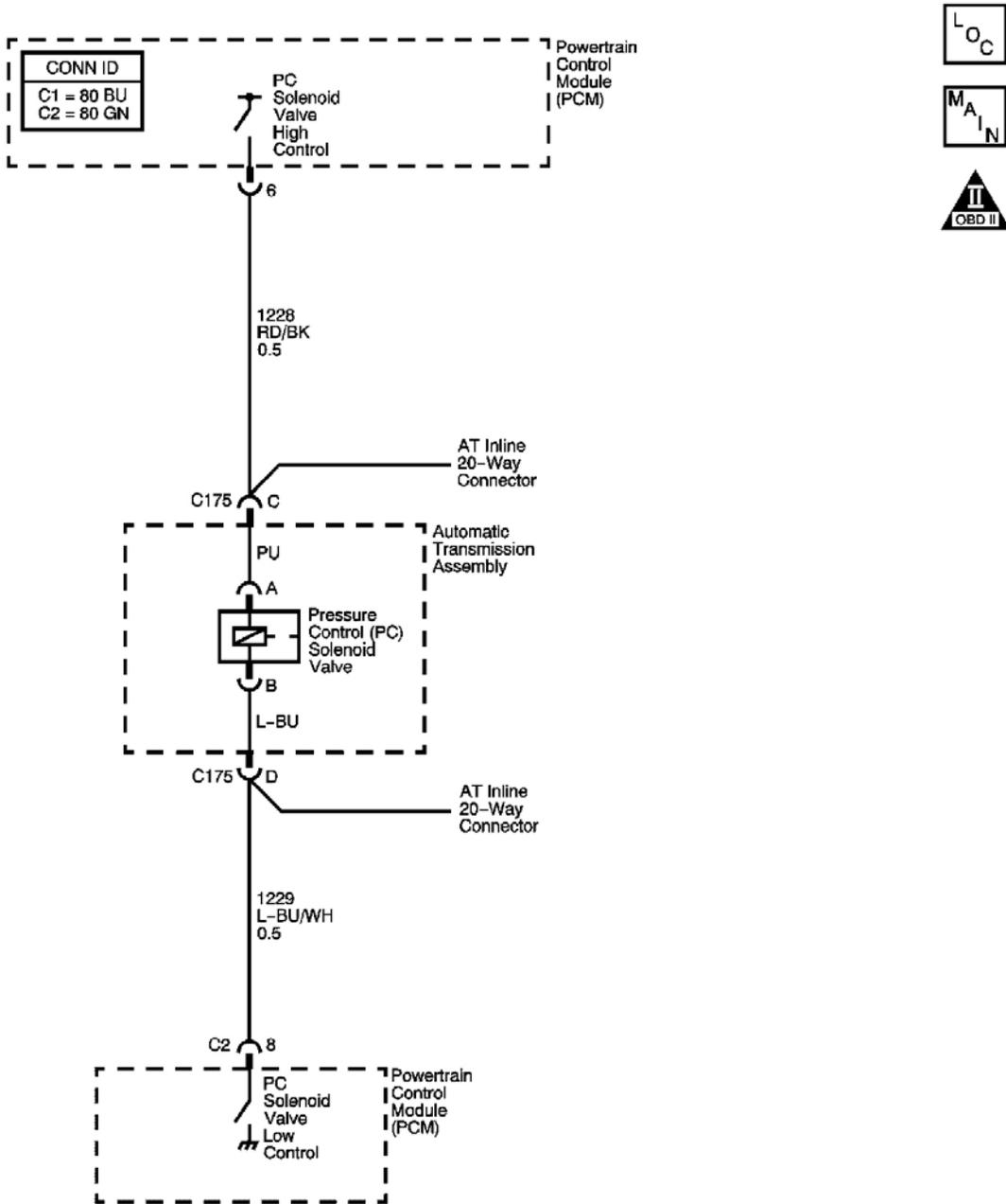
**Fig. 13: Pressure Control (PC) Solenoid Valve Diagram**
