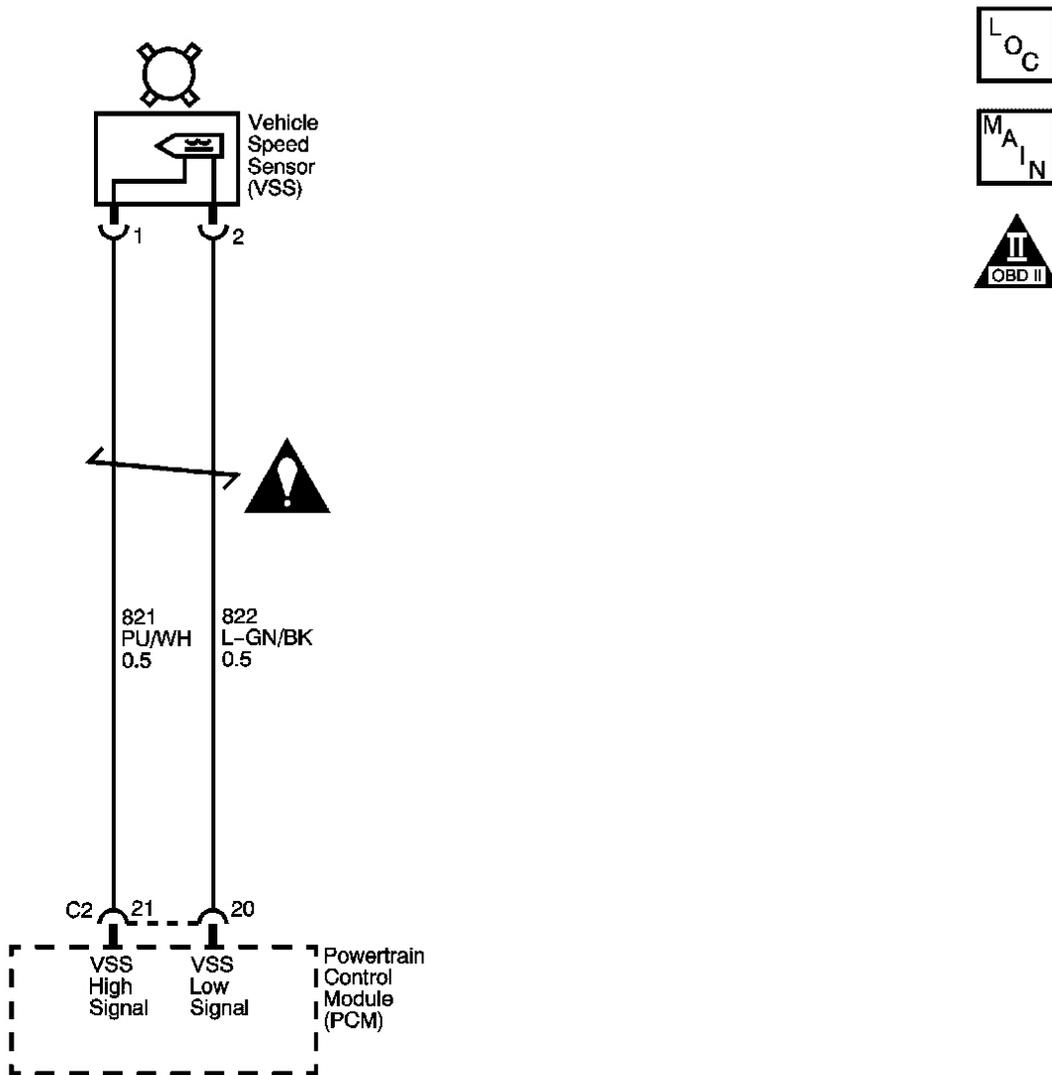
**Fig. 2: Vehicle Speed Sensor (VSS) Assembly Diagram**
