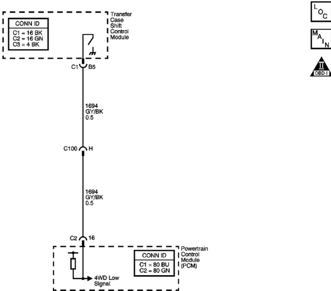
**Fig. 24: Four Wheel Drive (4WD) Low Circuit Diagram**
