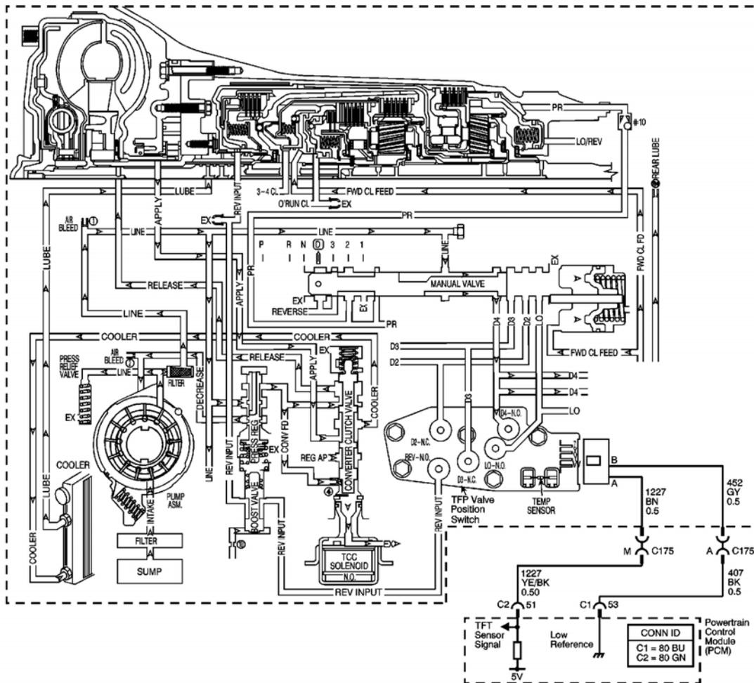
**Fig. 1: Filter, Control Valve Body Assembly, Transmission Case & Oil Pump Assembly**
