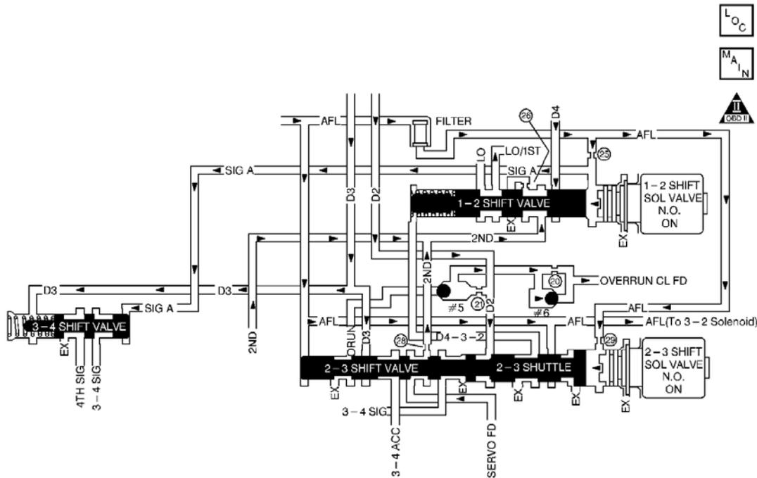
**Fig. 14: 1-2 Shift Solenoid (SS) & 2-3 Shift Solenoid (SS) Valve Fluid Diagram**
