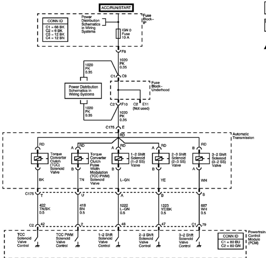
**Fig. 10: Torque Converter Clutch (TCC) Solenoid Valve Diagram**
