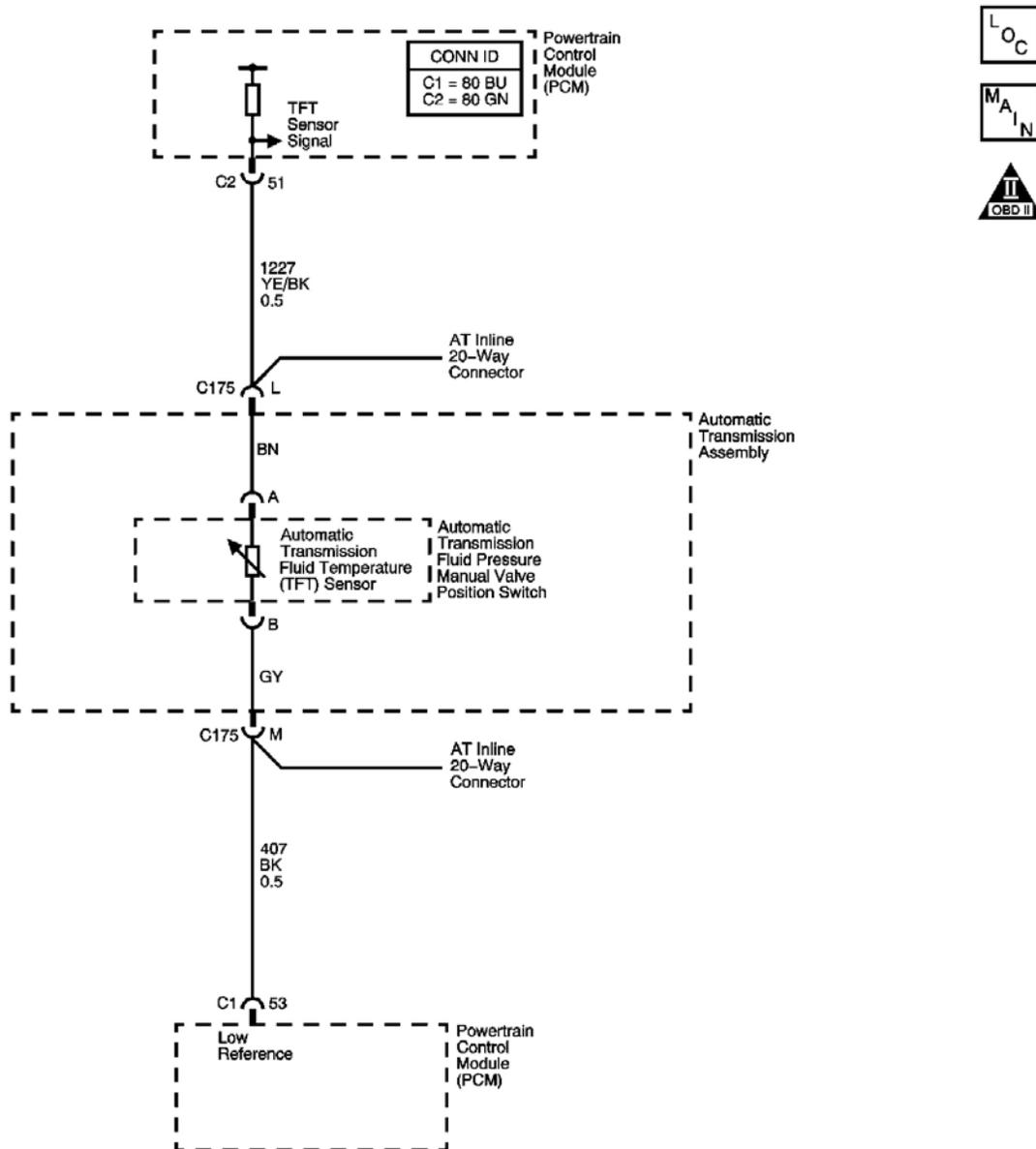
**Fig. 5: Automatic Transmission Fluid Temperature (TFT) Sensor**
