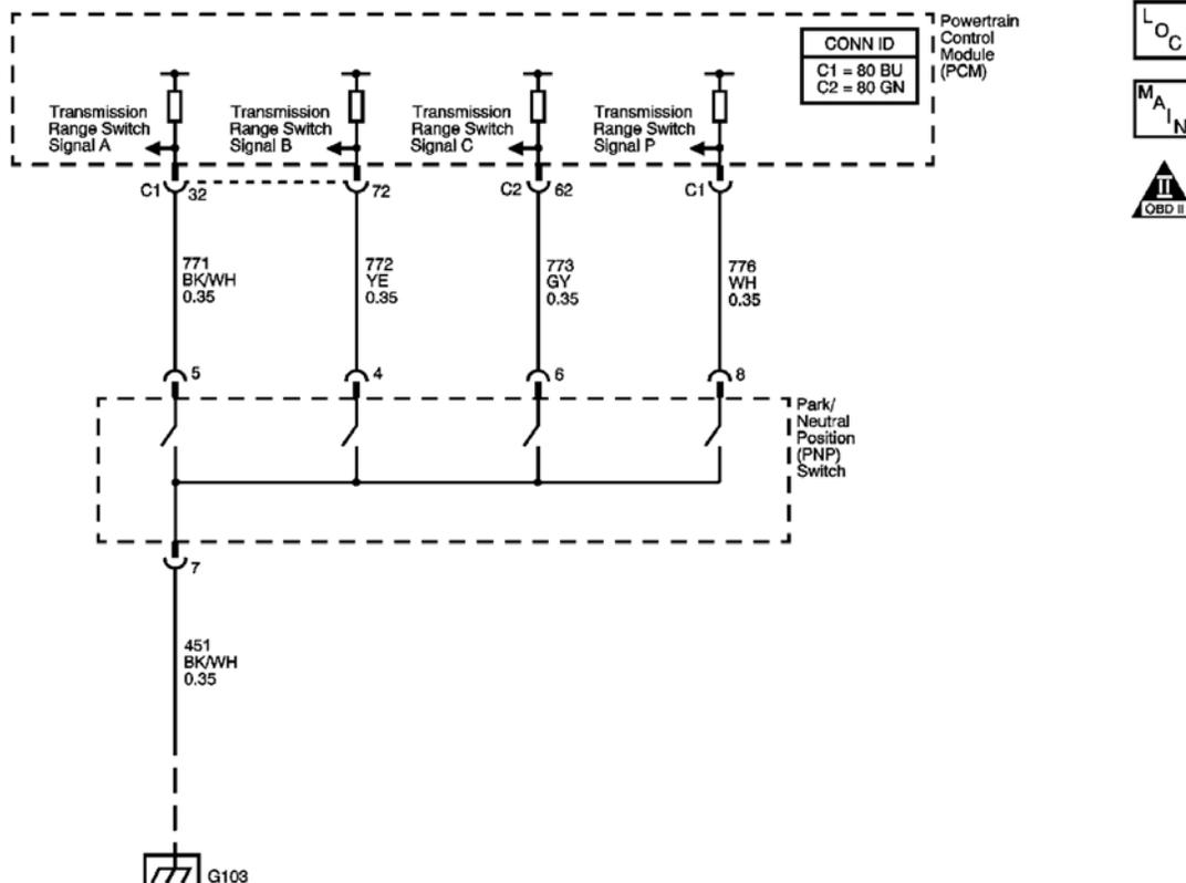
**Fig. 4: Transmission Range (TR) Switch Diagram**
